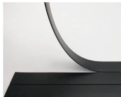
Removal of excess material on the pre-scored line
