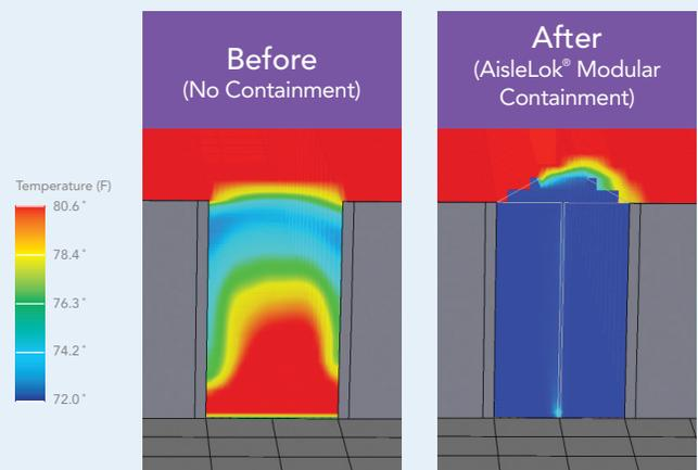
CFD Analysis shows hot air recirculation into the cold aisle.
