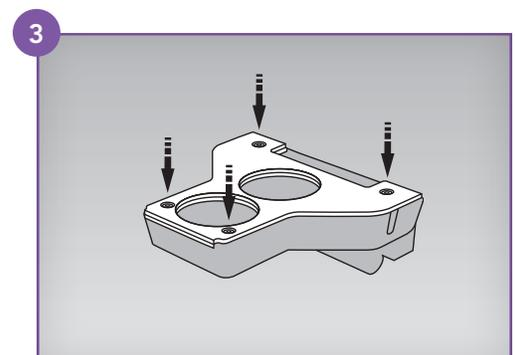
**PREPARATION:** Determine where the base plate will attach to the concrete floor. Align the side of the bottom plate that does not protrude past the vertical face of the post with a tile edge (or up against another surface, i.e., a wall), so the adjacent tile is not captured by the base plate. Be sure to use a vacuum to control dust and debris. Avoid using zinc coated hardware.
