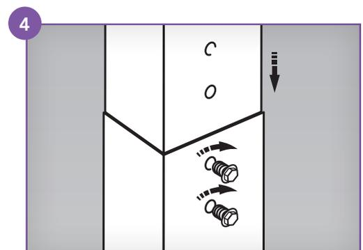
**REPLACING OF HINGE BACK PLATE:** The top hinge on the Bi-Directional Doors by design includes a Long Hinge Back Plate which attaches to the hanger bracket mounted to the top of a cabinet. When installing the AisleLok® Bi-Directional Doors to the Adjustable Mounting Post, this bracket will extend past the Adjustable Mounting Post. To prevent the extension from being an obstruction, replace the standard Long Hinge Backplate with the supplied Short Hinge Backplate.
